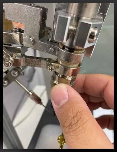
Once the soldering iron tip has cooled to room temperature, turn the nut at the red arrow (shown in the left image) clockwise to loosen it. No need to completely remove the nut; just loosen it until you can see the threads.
