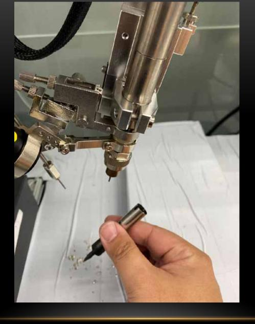
Finally, using your hand, apply force to pull the soldering iron tip downward to remove it.
