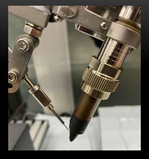
Continue feeding the solder wire until it is visible at the needle tip.
