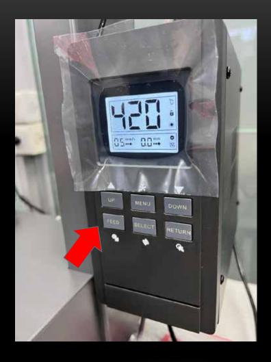
Turn on the soldering machine and perform a test (Press FEED ) to ensure the new solder wire feeds correctly and solder joints are formed properly.
