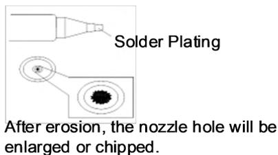
c. A layer of special alloy is plated inside and outside the nozzle aperture. If the alloy layer is eroded due to high temperature, the nozzle will not be able to maintain a proper temperature.
